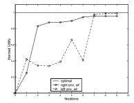
Figure 3. The performance of online policy iteration for wall following in two environments
